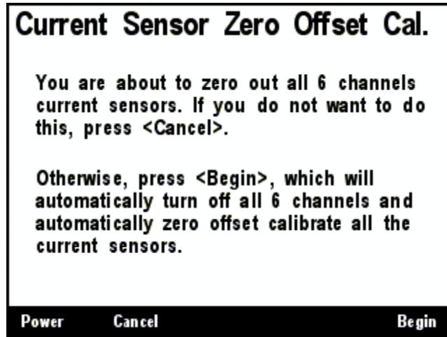
Figure 57 – DCR100 Current Sensor Zero Offset Calibration Screen
